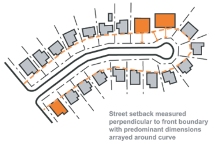
Figure 3.2.5.3 Building frontage setbacks - curvilinear street
