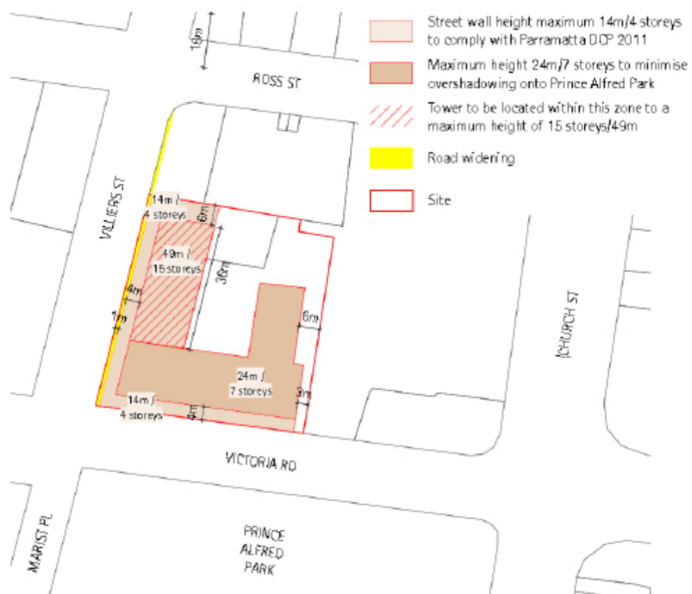
Figure 4.3.3.7.22 Built Form Design Controls – Heights and Setbacks
