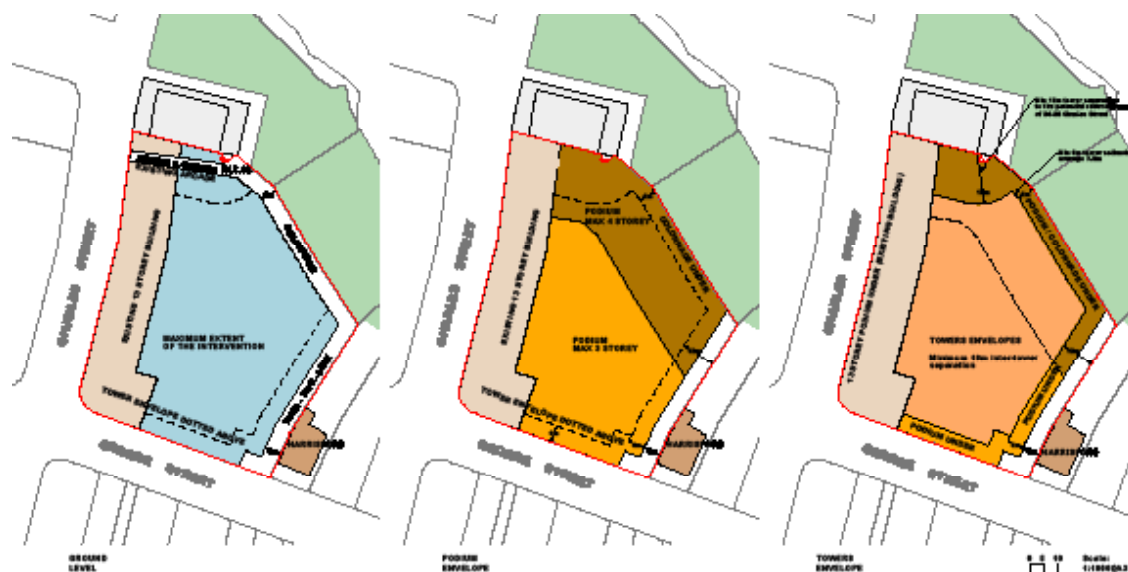
Figure 4.3.3.7.26 Building heights, setbacks and envelopes
