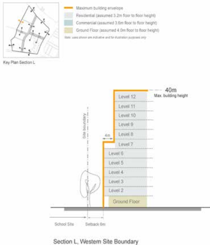
Figure 4.3.4.1.15 Indicative Site Sections
