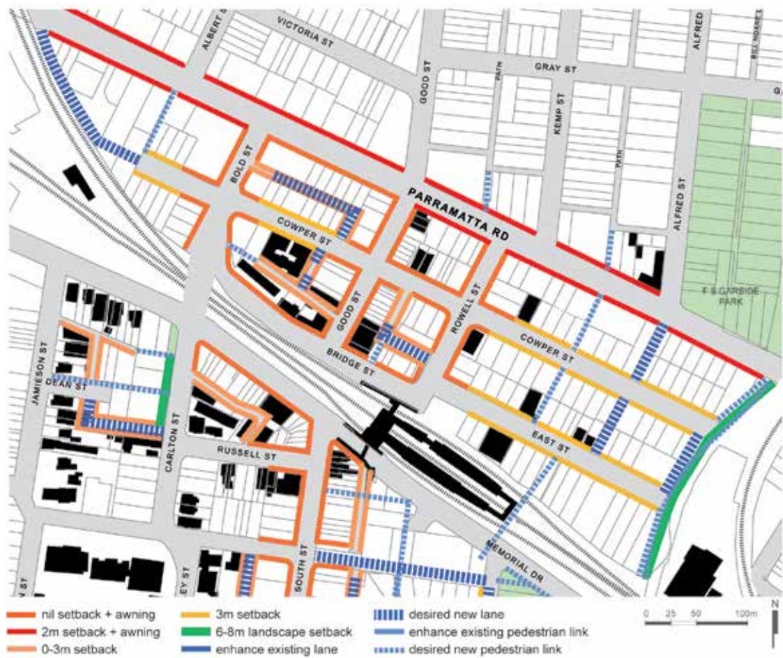
Figure 4.1.6.3 Building Setbacks, Pedestrian Links and Laneways
