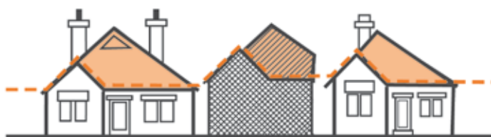
Figure 3.2.3.1 Sympathetic and complementary roof designs
