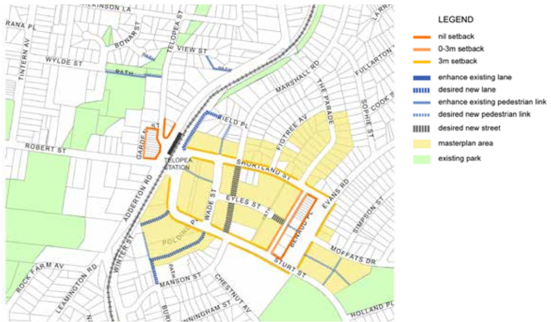
Figure 4.1.11.2 Building Setbacks, Laneways and pedestrian links
