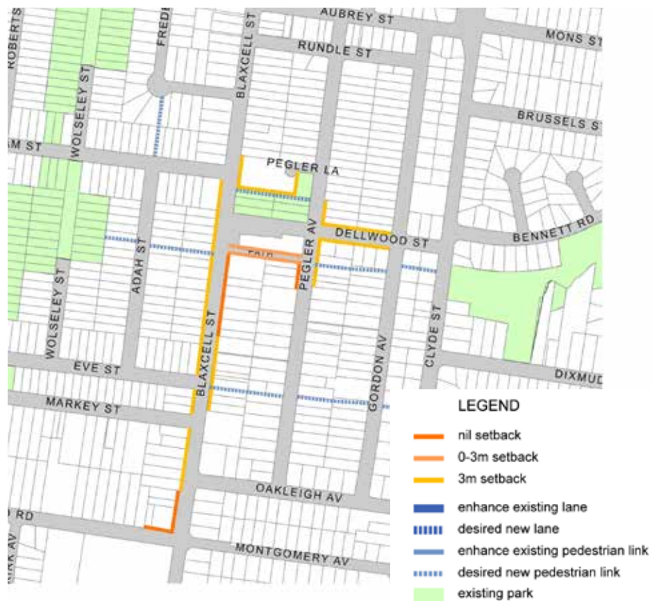
Figure 4.1.10.2 Building setbacks, laneways and pedestrian links
