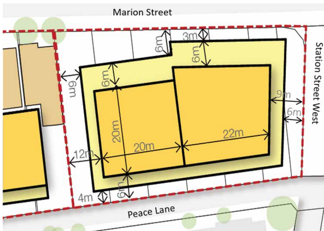
Figure 4.3.3.7.70 Building alignment and setbacks
