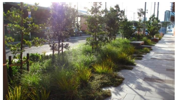
Figure 12 Bioswales could be located in streetscapes to improve the water quality in the precinct
