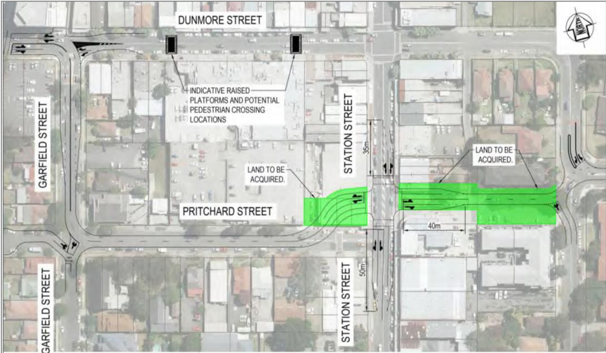
Figure 11: Full bypass option - as contained in the Traffic and Transport Study (source: Bitzios Consulting)
