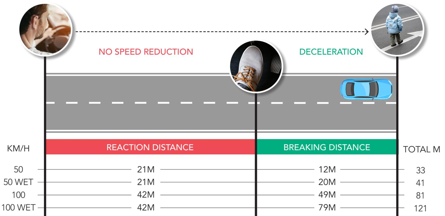
When driving 50 km/h your vehicle moves 13.9 m every second. With an average driver reaction time of 1.5 seconds, driving 50 km/h you'll have travelled 21m **just reacting on danger** (first example shown above). This is why a 3 second following distance is essential, in case of an emergency stop. If weather conditions change from dry to wet, you will need to leave an even larger following distance.
