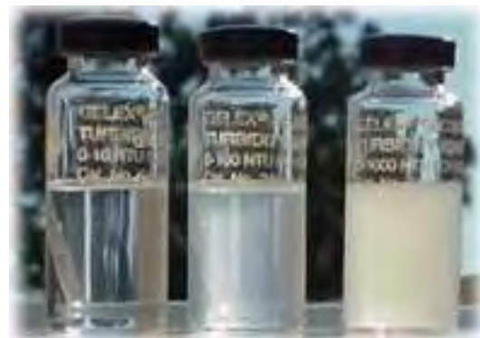
Figure 15: Visual relationship between 5 NTU (LHS), 50 NTU (centre) and 500 NTU (RHS).
