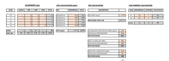
Figure 4- Proposed apartment mix and other calculations for Site 1
