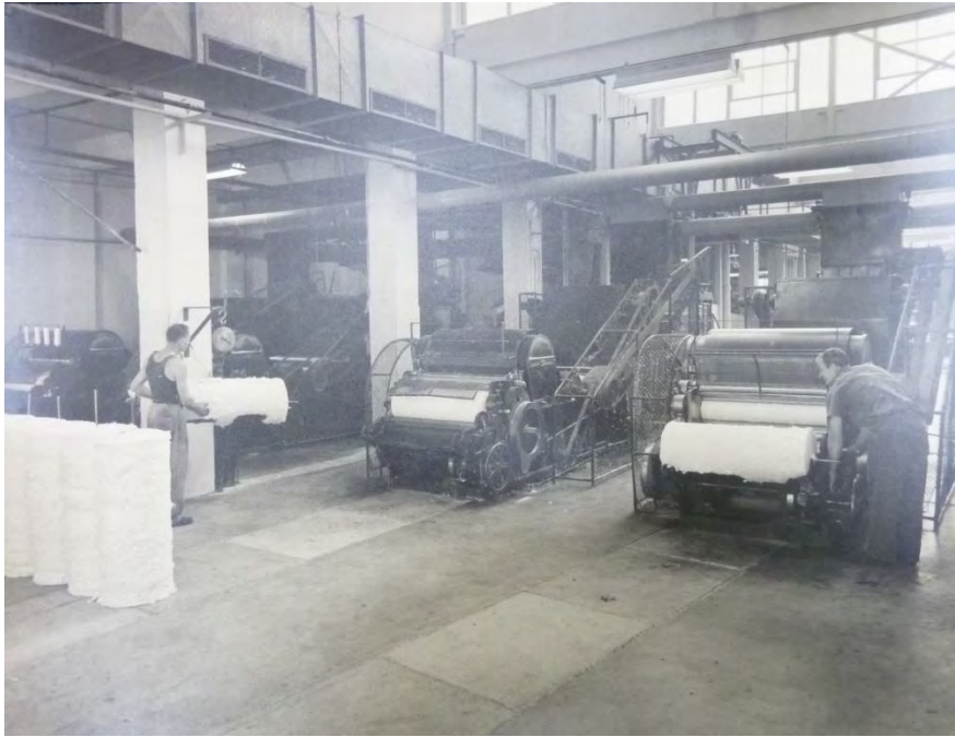
Figure 39 Producing the laps, rolls of exactly 40 yards in length, which are weighed on the scales at left for uniformity and weight per yard, vital for producing an even-textured, super quality yarn. (Source: Pacific Brands archives)
