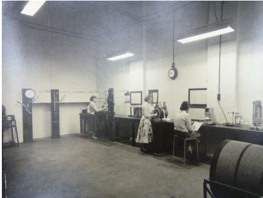
Figure 45 The Testing Laboratory where yarns were tested for various parameters including strength. Some of the testing equipment survives as movable heritage. (Source: Pacific Brands archives)
