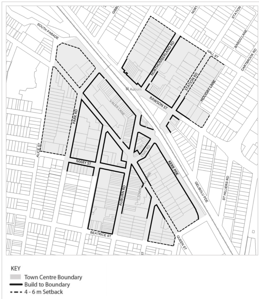
Figure 2: Building setbacks within the Auburn Town Centre
