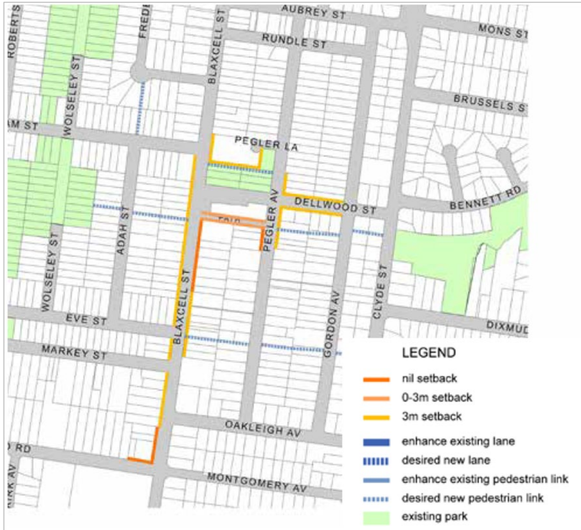
Figure 2: Building setbacks, laneways and pedestrian links
