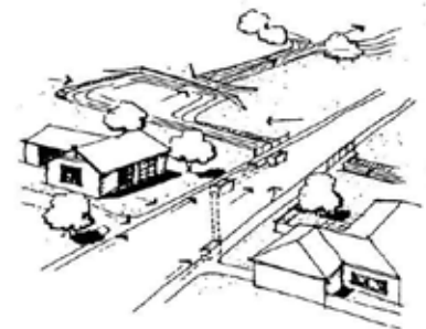
Figure 5: Typical combination of public roads, piping, retention basin and stream.
