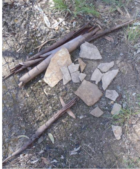
Photo 2 – Asbestos Cement Fragments at TP30
