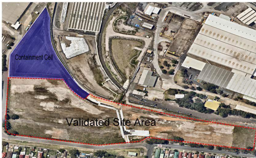
Figure 22. Aerial view of Lot 12 showing the previously remediated (validated) site area and the containment cell (Source: DLA LUSR)
