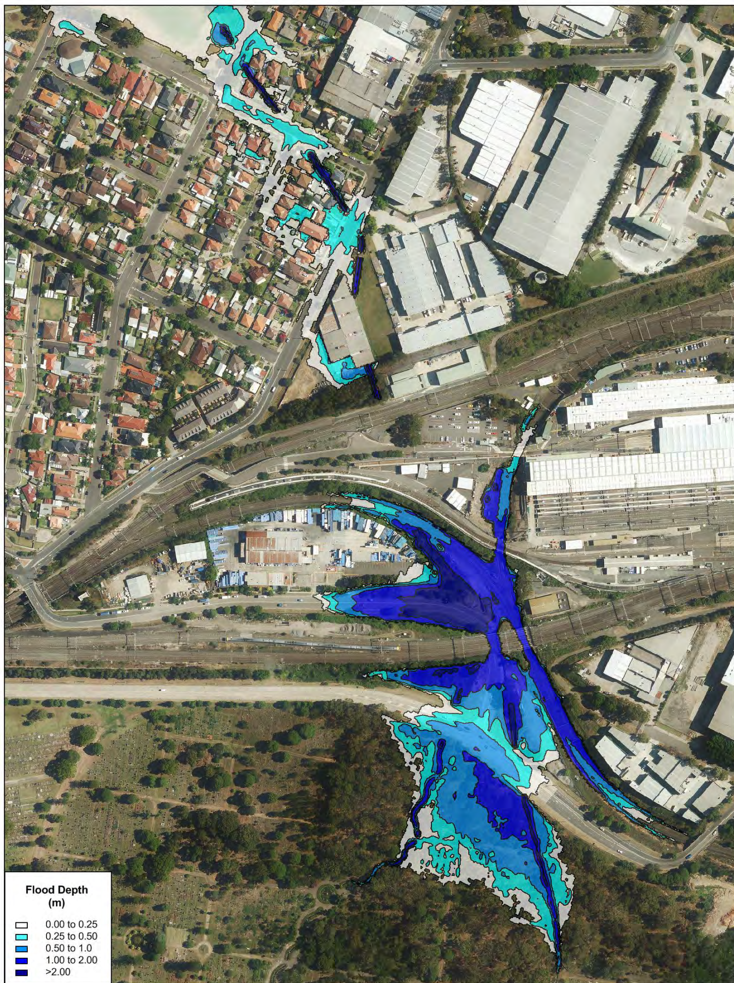
FIGURE B3 Existing Scenario - 1% AEP + Climate Change Flood Depths
