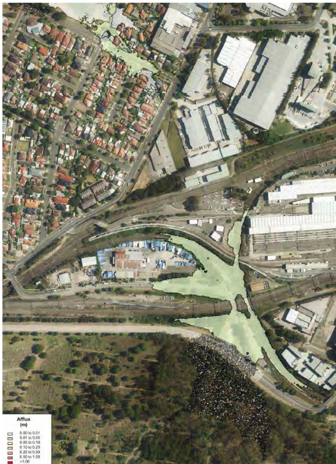
Plate 5-4 – Impact Plot: Change in 1% AEP Flood Depths
