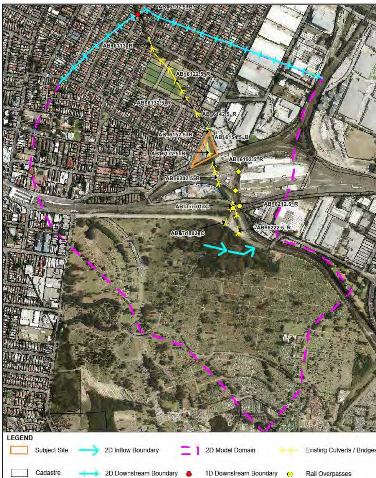
Plate 4-1 – Model domain, boundary conditions and key structures
