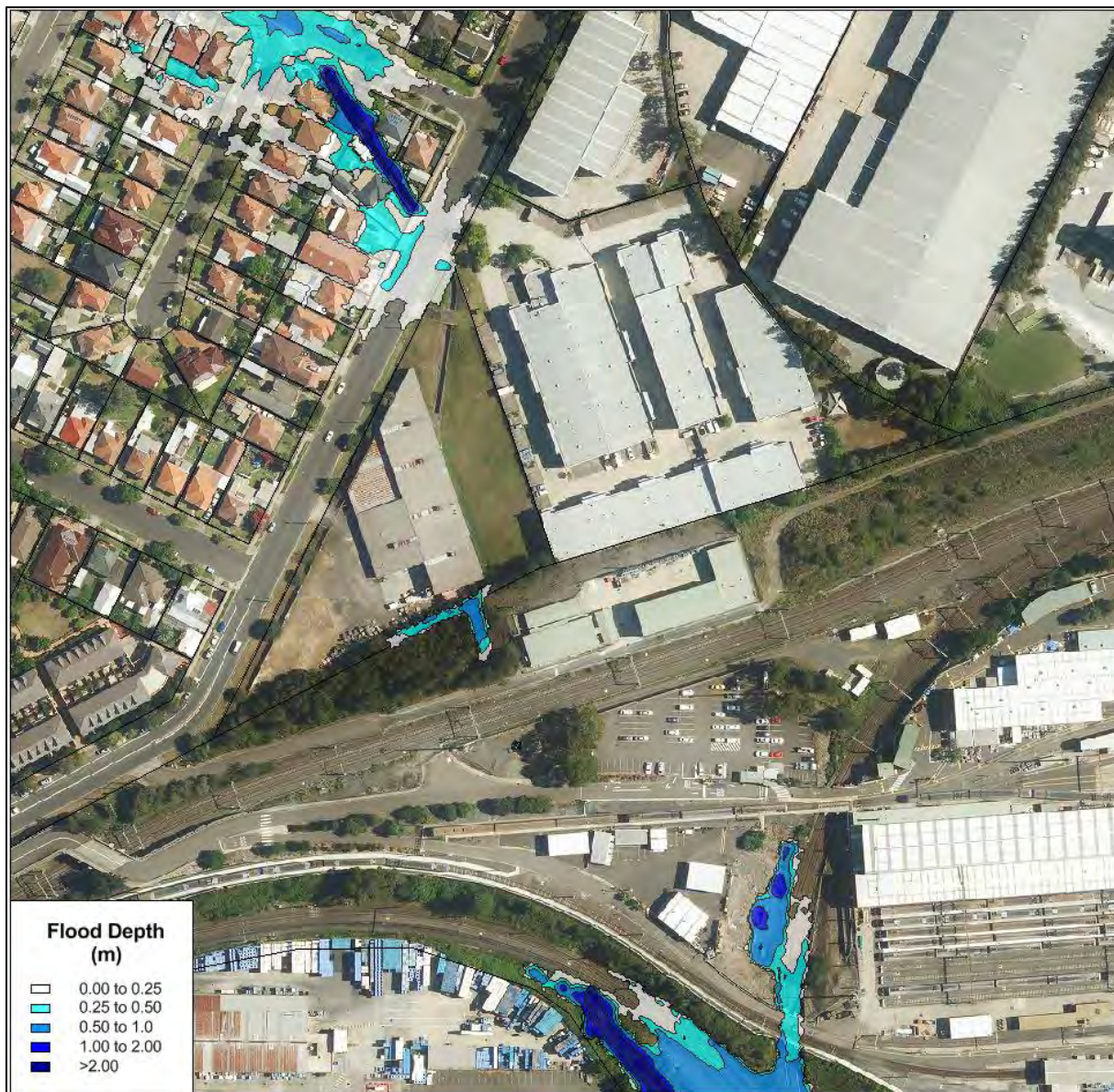
Plate 5-6 – Design conditions flood depth plot 1% AEP event – TestCase2
