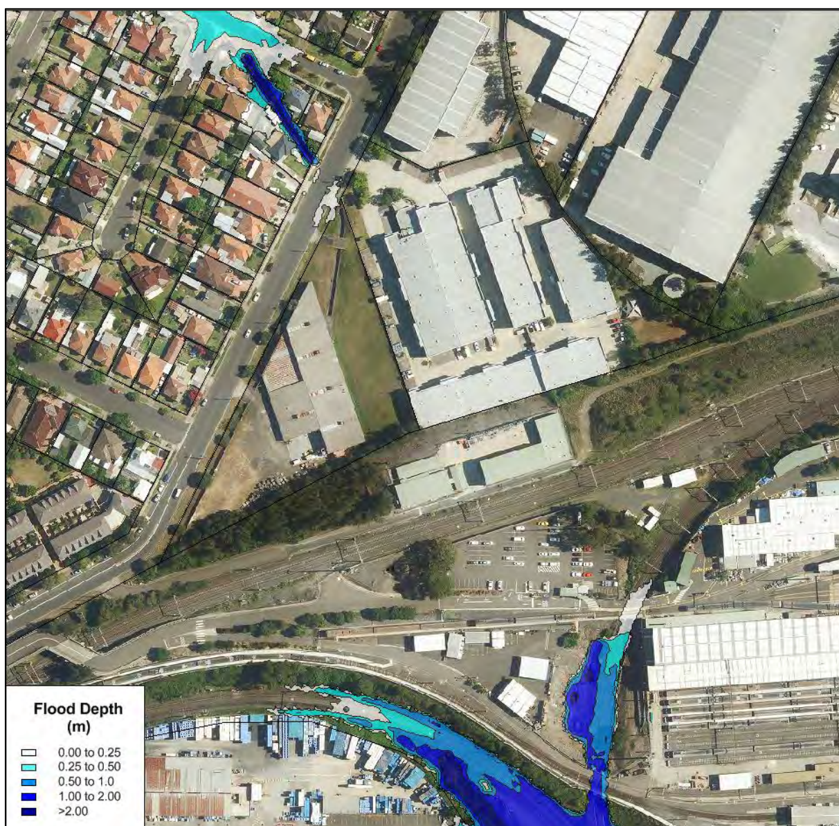
Plate 5-3 – Design conditions flood depth plot 1% AEP event
