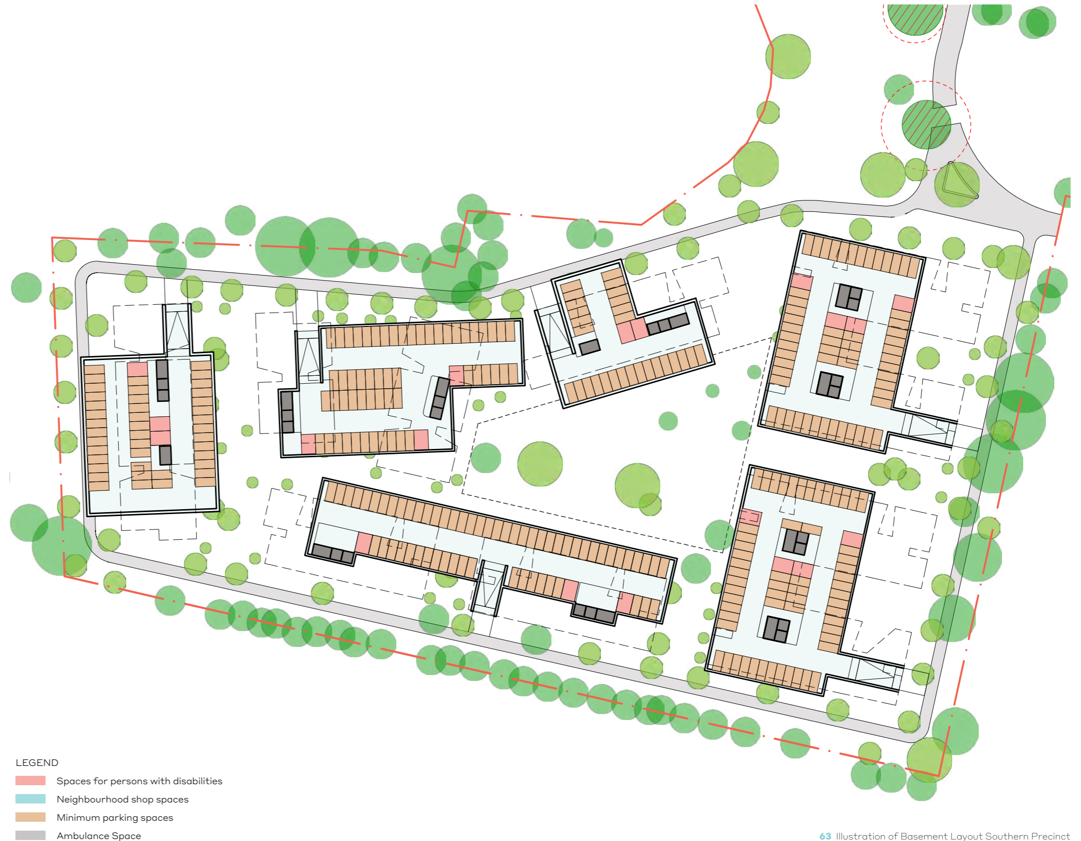
63 Illustration of Basement Layout Southern Precinct
