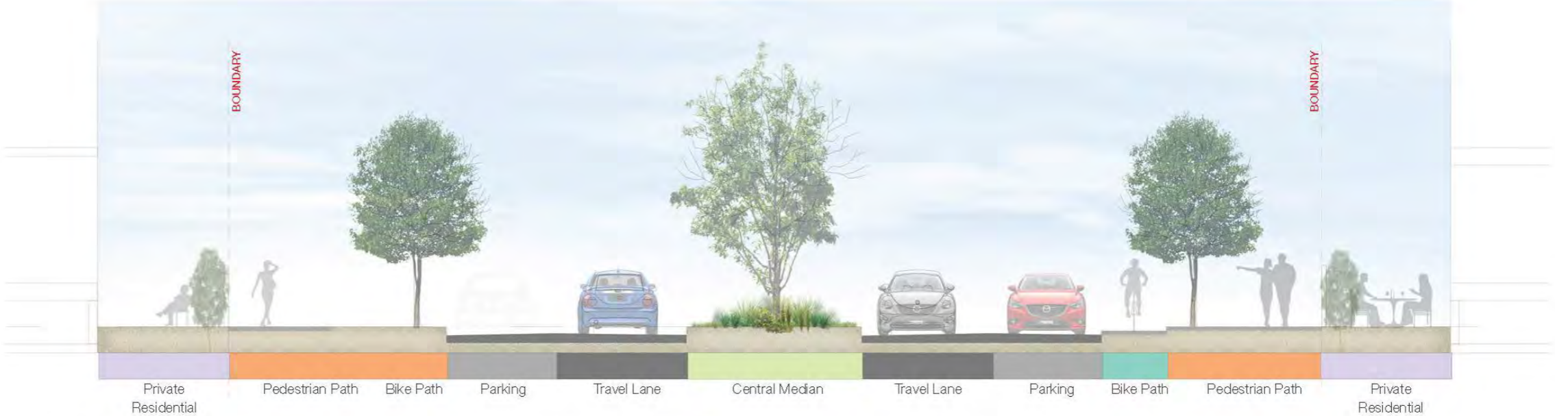
Section BB Proposed Option 1 - Central Median (Used in Concept Masterplan)
